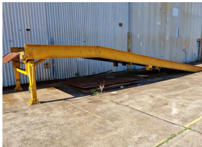
Figure 5.1: Example of external loading dock ramp
