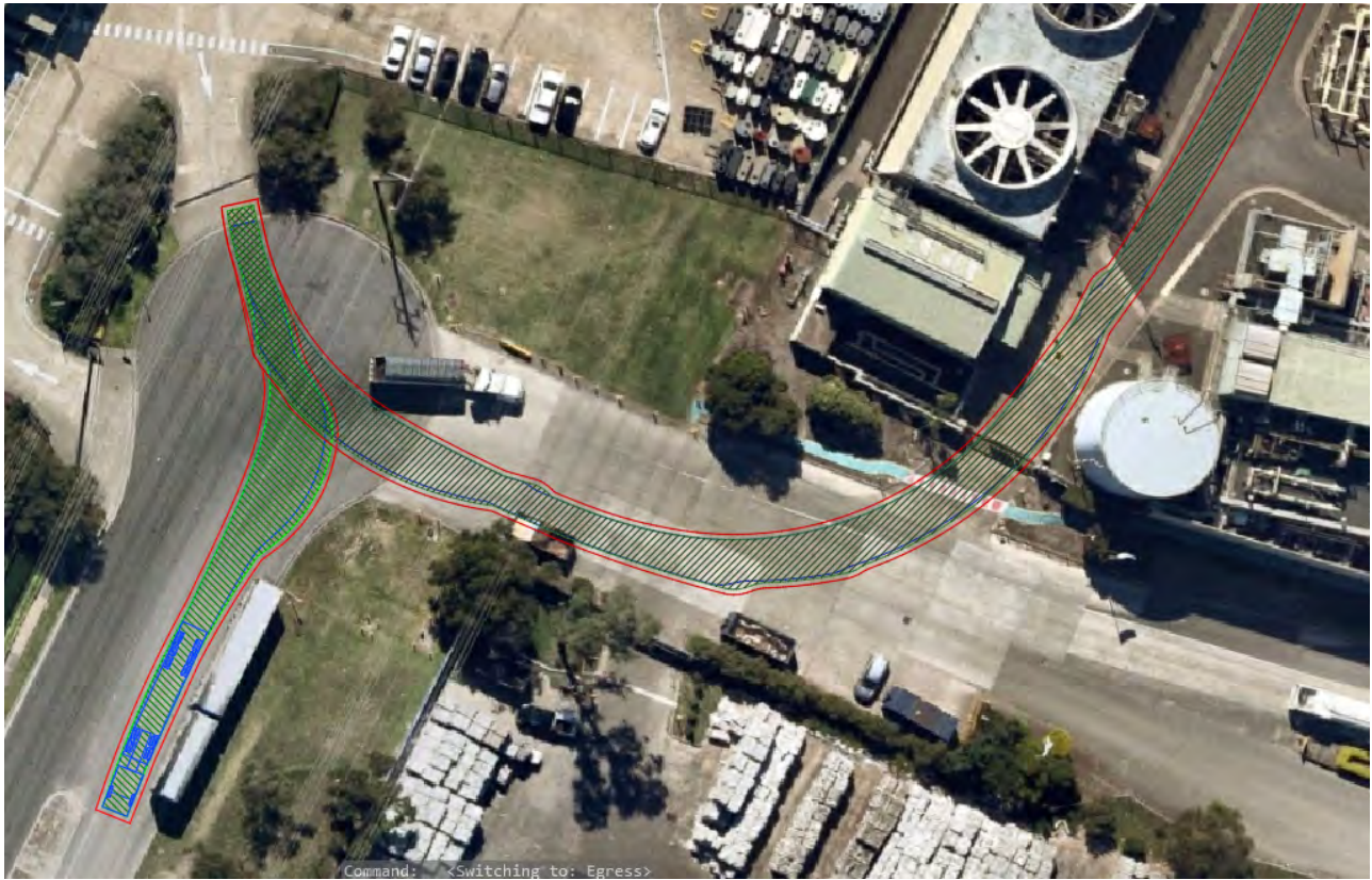
Figure 5-2 Egress of the 19 metre six-axle vehicle
