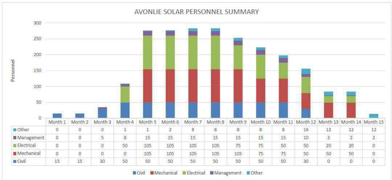
Figure 4-1: On-site workforce over construction period (Source: Avonlie Vehicle and Personnel Summary Rev C, SGRE)
